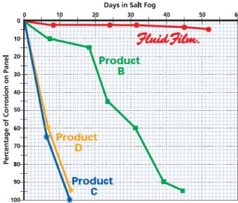
Testing was performed in the laboratory of Eureka Chemical Company according to procedures similar to ASTM methods for measuring corrosion.
